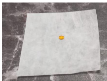
Fig. 1 Hydrophobic polypropylene substrate (N_control) and a water droplet
